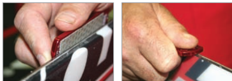
Removing cuts in edges with a diamond stone
