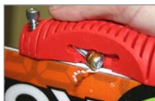
Removing sidewall offset
